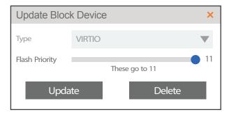
HC3 has built-in, real-time IOPS meters for each virtual disk so the results of changing the priority on a particular disk can begin to be seen immediately. Because the virtual disks can be changed dynamically, the priority can be adjusted as much as necessary to achieve the correct balance of IOPS efficiency across virtual disks and VMs.
